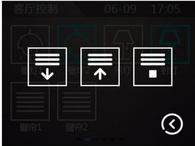
Depending on the configuration of the software parameters, in blinds/curtains mode, two or three buttons can be invoked;
