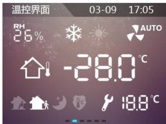
The top row: humidity, cooling, heating, speed, speed status
