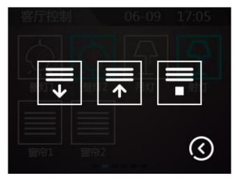
Depending on the configuration of the software parameters, in blinds/curtains mode, two or three buttons can be invoked;
